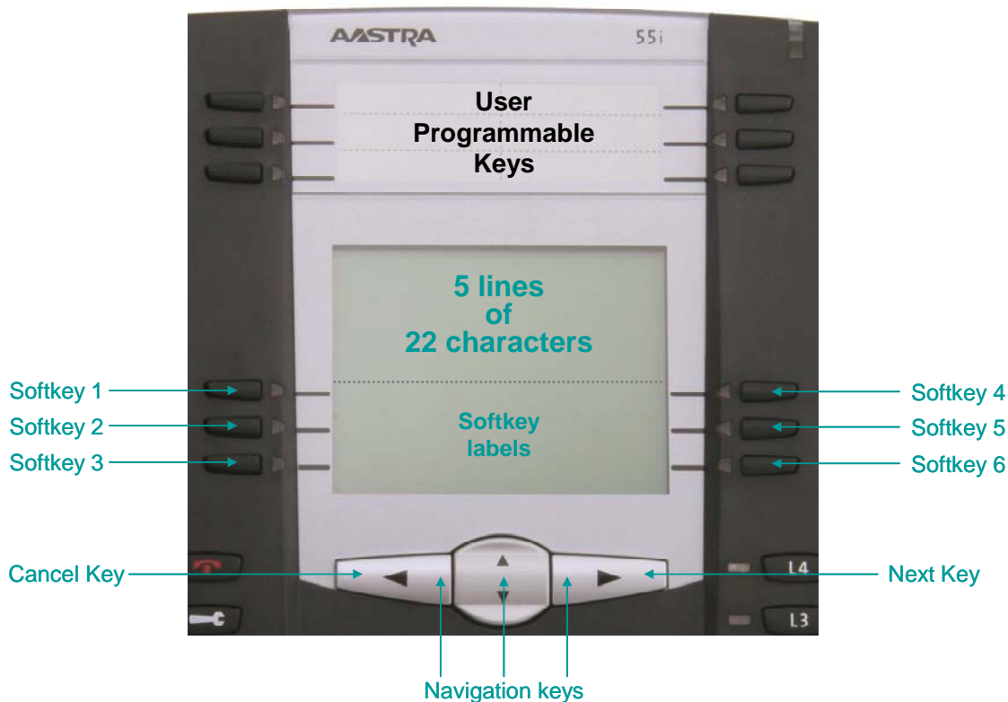
Figure 10: Aastra 55i XML display and keys
